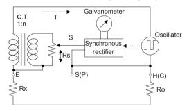
Measurement principle diagram (2-pole measurement)
