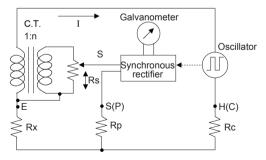
Measurement principle diagram (3-pole measurement)
