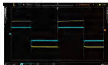
Linear CC mode, PWM 10A 250Hz
