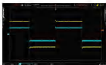
Linear CC mode, PWM 10A 2.5Hz
