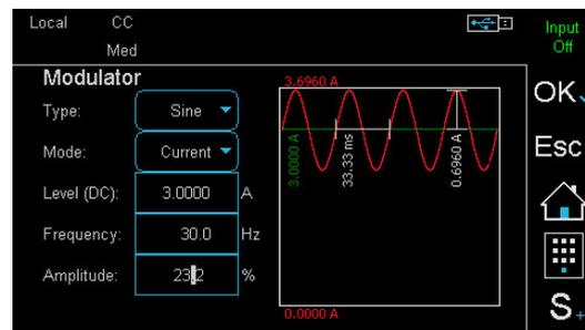
The modulator adds a sinusoidal, square-wave or triangular signal to a static setting in CC or CV mode. Frequency and modulation depth are adjustable.
