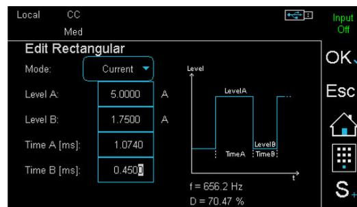
The rectangular function provides a convenient way to generate a rectangular waveform by entering absolute time and amplitude values.
