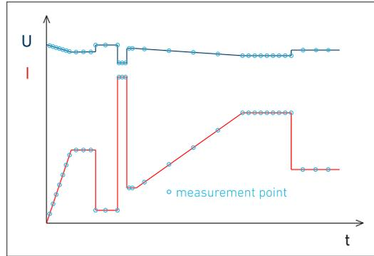
Load profile generated by List function with synchronized data acquisition of time, voltage, current
