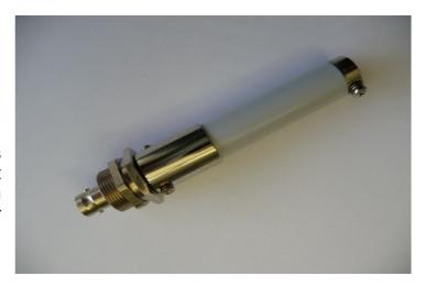
The Broad-band pulse voltage divider, type PVD is a state-of-the-art measuring equipment whose excellent high-frequency transmission characteristics can be fully exploited only if properly operated and if all aspects typically encountered in the sub-microsecond time region, e.g. appropriate grounding, transmission line characteristics of leads, are fully considered.
