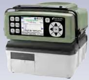
**Service Module:** allows for general maintenance and can be used as an alternate source of vacuum during stationary operation.
