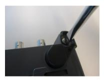
**4.** Detach the hardware module(s) from the MT1000A controller, then attach the handgrip to the controller. The handgrip can be placed on the left or the right side of the instrument, whatever your preference.
