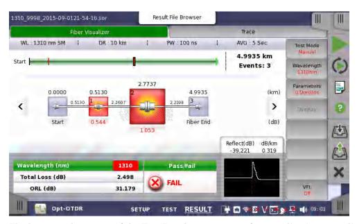
The layout and contents of the Test Results screen vary from application to application. There may be a vertical menu of soft keys on the right side, where you can change parameter values before re-running the test (green arrow icon on the Application toolbar). To save results to a file, touch the **Download** icon on the Application toolbar.
