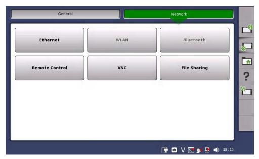
**Ethernet** lets you set up the instrument for Ethernet connection, either via dynamic addressing (DHCP) or manual specification of IP address, subnet mask, and default gateway.
