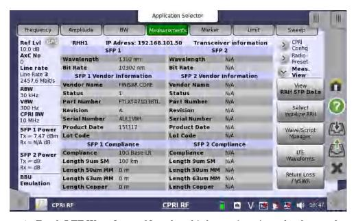
**9.** Touch **LTE Waveforms**. Note that this button is active only after you have initialized the RRH in the preceding steps.
