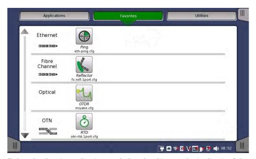
To launch a favorite application, touch the related icon on the Application Selector Favorites screen. The port resources associated with the application when the favorite was created are automatically allocated and the saved settings are loaded. If the designated resources are not available, you will be prompted to select alternative port(s).
