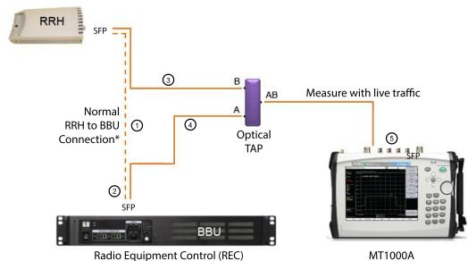
\* Lock down the Radio before disconnecting fiber from BBU
