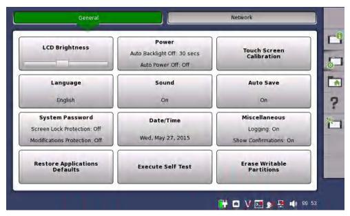
LCD Brightness lets you adjust the screen brightness by dragging the slide bar.
