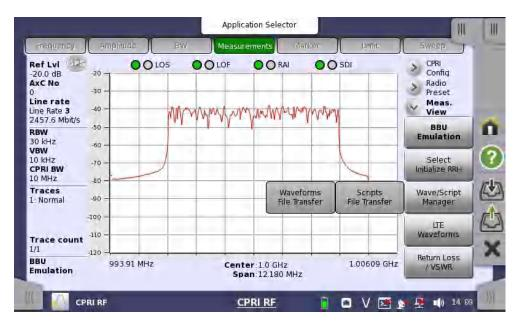
**4.** In the File Transfer dialog, navigate to the appropriate folder on the USB device, then select the scripts and touch the black arrow to copy.
