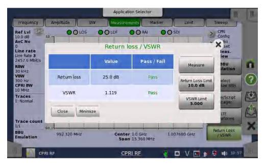
**19.**You can optionally change the return loss limit and VSWR limit and press **Measure** to run the test again.
