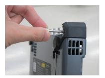
7. Attach the last module with rear cover and tighten the corner screws.
