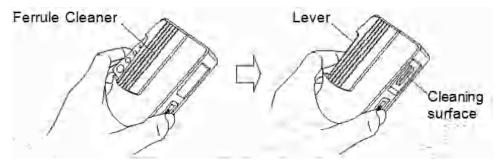
**2.** Hold the lever in the open position and push the connector ferrule tip into the cleaning surface, swiping the connector to clean.
