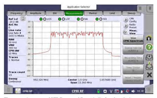
The connection status of SFP Port 1 and Port 2 is displayed on the instrument screen, above the trace window. Green indicates a good connection, red indicates an error, and gray (no color) means no connection. In the example above, Port 2 has no connection.
