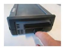
**3.** Lay the instrument face down on a flat surface and remove the screw from each of the four corners.
