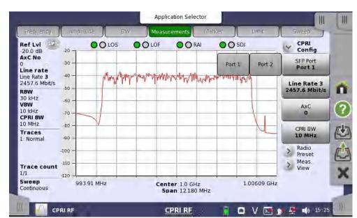
2. Select the SFP port to which the CPRI link you want to monitor is connected.
