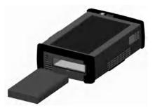
**6.** When inserting the battery pack, note the position of the battery terminals. With the instrument screen facing up and the battery compartment towards you, the terminals should be in the upper left corner.
