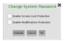
In the dialog box that follows, you can optionally enter a new password in the text field. Your key input is masked by default. To see the characters as you type, select the Display Password checkbox. Touch **Cancel** to keep the current system password.
