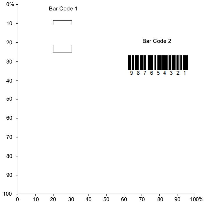
**Note:** A bar code needs only to be touched by the centering window in order to be read. It does not need to pass completely through the centering window.
