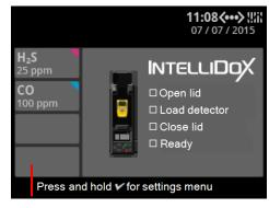
Multi-inlet key: IntelliDoX activates gas inlets 1, 2,
