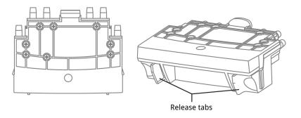
Insert the single-inlet key when only one gas inlet is required to support compliance test operations performed on the module.
