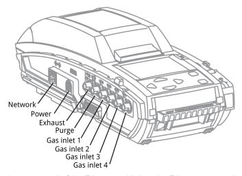
Insert one end of the Ethernet cable into the Ethernet port on the module. Insert the free end of the Ethernet cable into the network outlet. When the module is connected to the network, the network symbol is displayed at the top right corner of the LCD.
