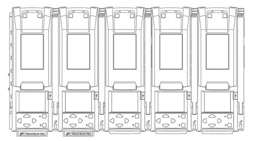
Up to five modules may be connected to form a group. Connected modules share the power supply, exhaust tubing, inlet filter, connected test gas cylinders and network connection. Follow these steps to assemble and prepare groups of up to five connected modules for first use:
