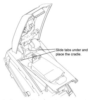
8. Use a screwdriver to fasten the two screws on the replacement cradle.
