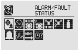
Figure 161. Alarm/Fault Status screen
