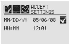
Figure 71. Accept Time-Date Changes screen
