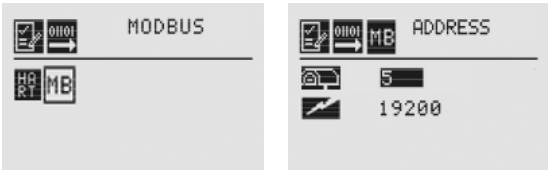
Figure 182. Modbus Configuration Display screen
