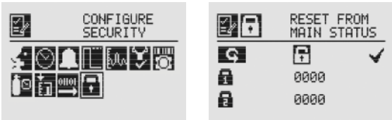
Figure 141. Configure Security screens
