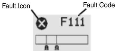
Figure 12. General Status Fault detail
