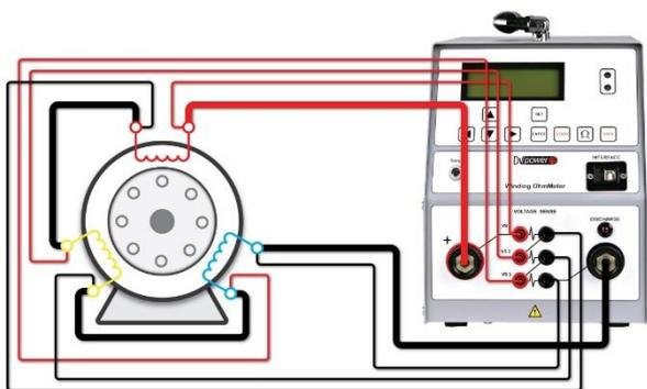
This way, all windings are externally connected in series and individual windings resistances are being measured. This measurement method is much faster than the previously explained one since the winding saturation process is performed only once.
