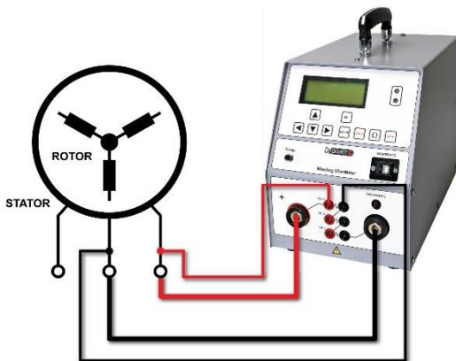
It is possible to measure motors' and generators' winding resistance in all phases at the same time. This is achieved by using three voltage sense channels and it is possible when all connection points of stator windings are accessible.
