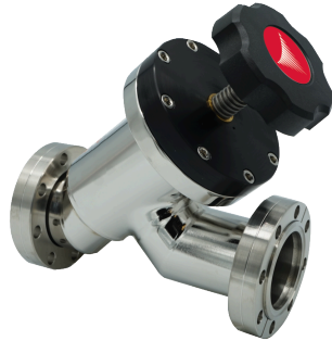
UHV inline valve, DN 40 CF, manual, SS/Cu/FKM, "A"-dim. 133 mm
