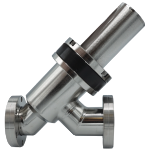
UHV inline valve, DN 40 CF, electro-pneumatic, PV 24 V DC, SS/Cu/FKM, "A"-dim. 133 mm
