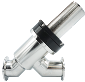
HV Inline valve, DN 16 ISO-KF, electro-pneumatic, PV 24 V DC, SS/FKM, "A"-dim. 102 mm
