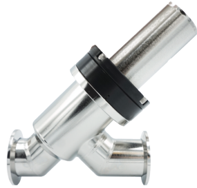
HV Inline valve, DN 50 ISO-KF, pneumatic, SS/FKM, "A"-dim. 178 mm
