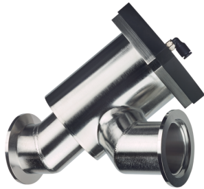
HV Inline valve, N-series, DN 50 ISO-KF, electro-pneumatic, PI (PNP)/PV 24 V DC, SS/FKM
