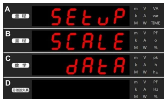
Figure 6.24 Set external VT/CT proportional constant
