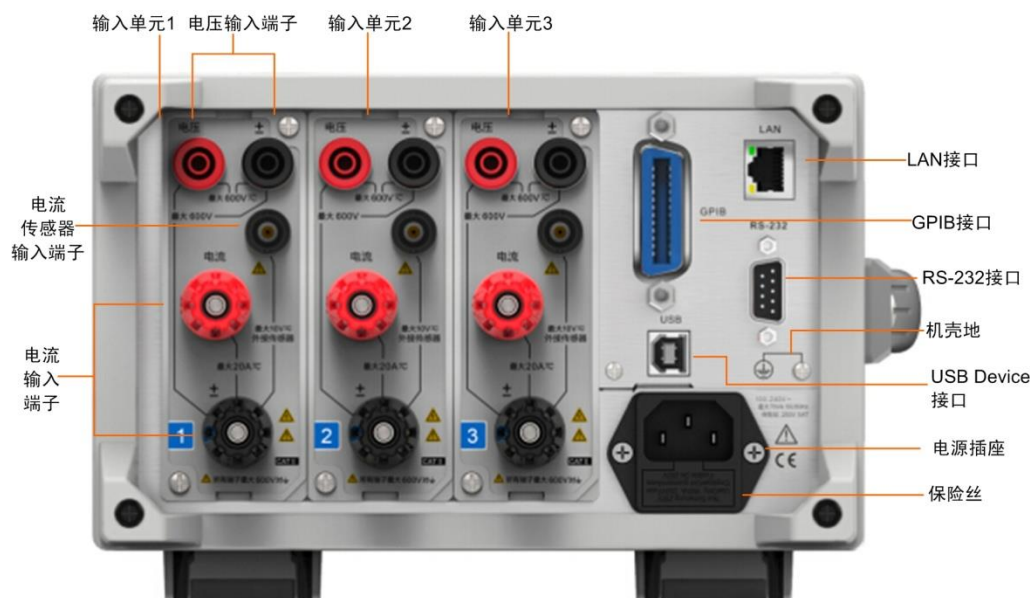
Figure 3.23 Rear panel description of PA323 power meter
