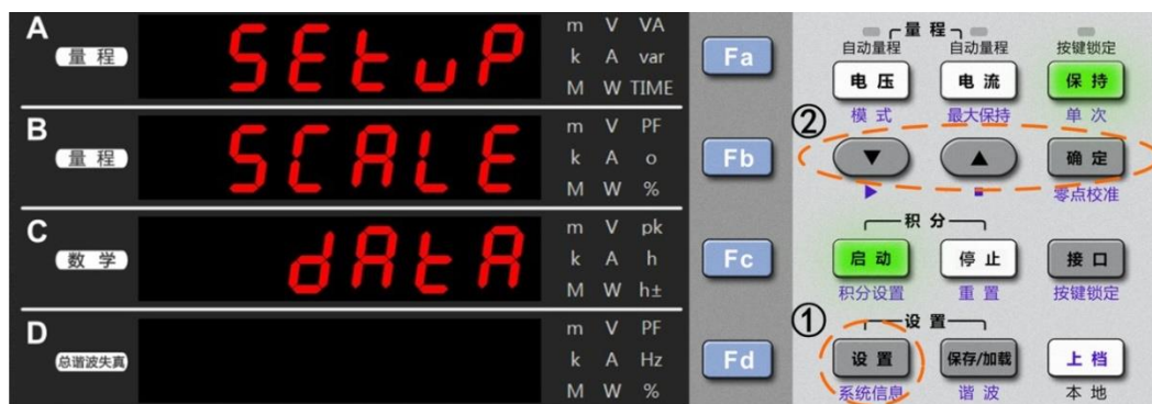
Figure 6.20 Set external VT/CT proportional constant
