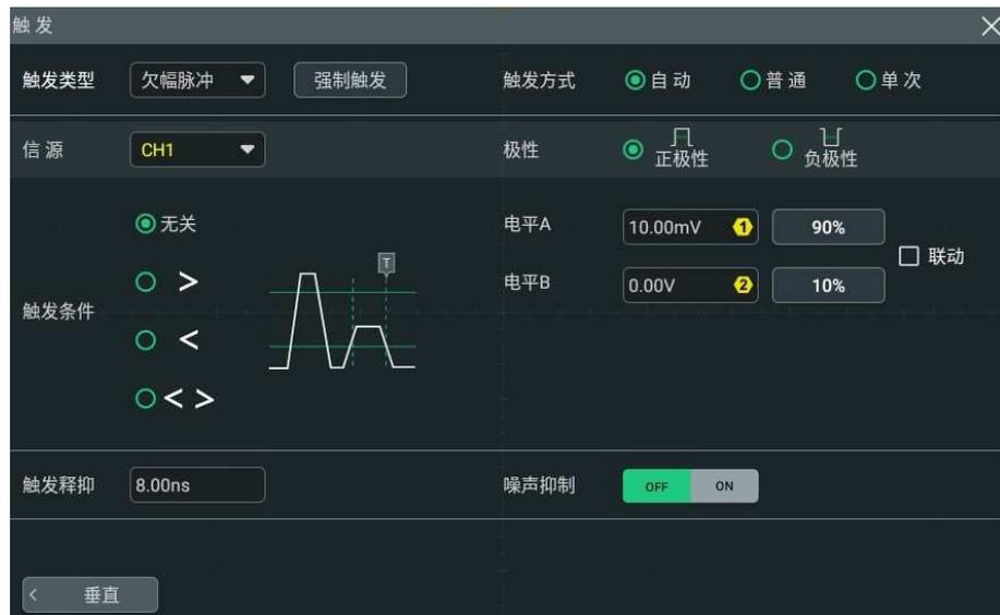
图 8.16 欠幅脉冲触发配置菜单
